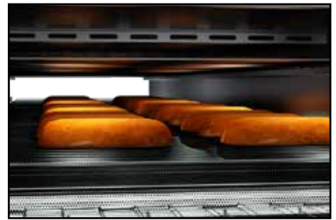
The perforated steel belt is used for free-form, high-rise loaves and the like.
